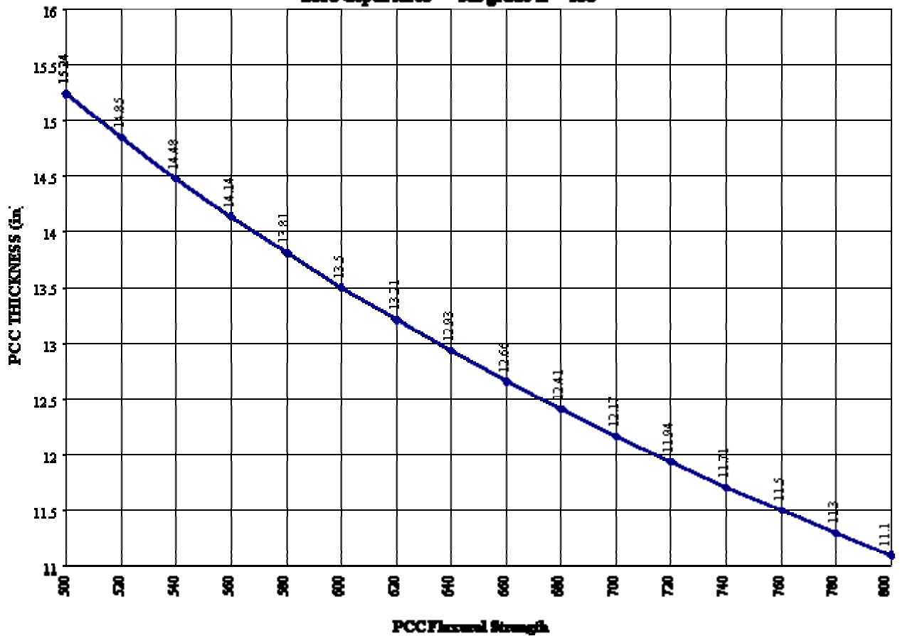
Required thickness for DUAL, WE-100 at 125000 lbs k on top of all subbase = 280 pd 2016 departures – sub grade k = 100
