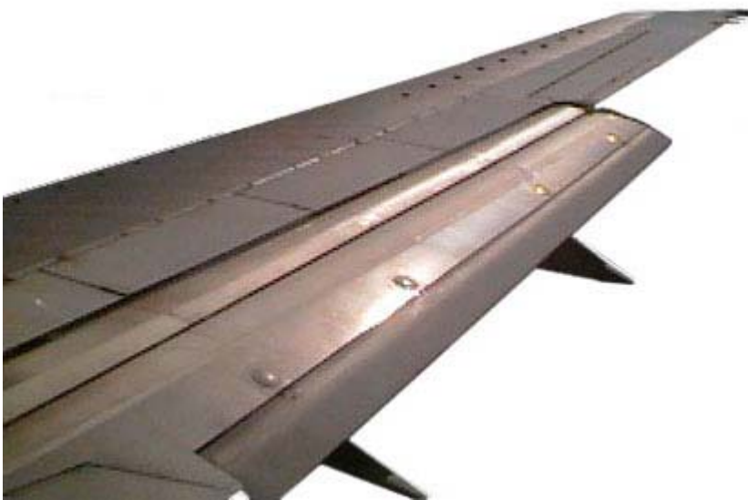
Figure 2. The triple-slotted flap system used on a 737.
