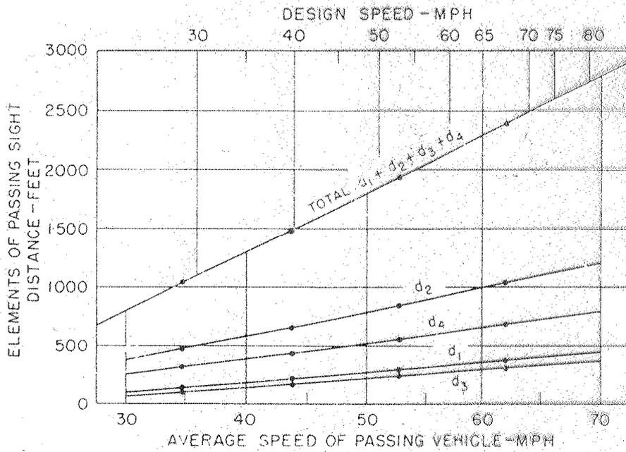
Figure III-2. Elements of and total passing sight distance—two-lane highways.
