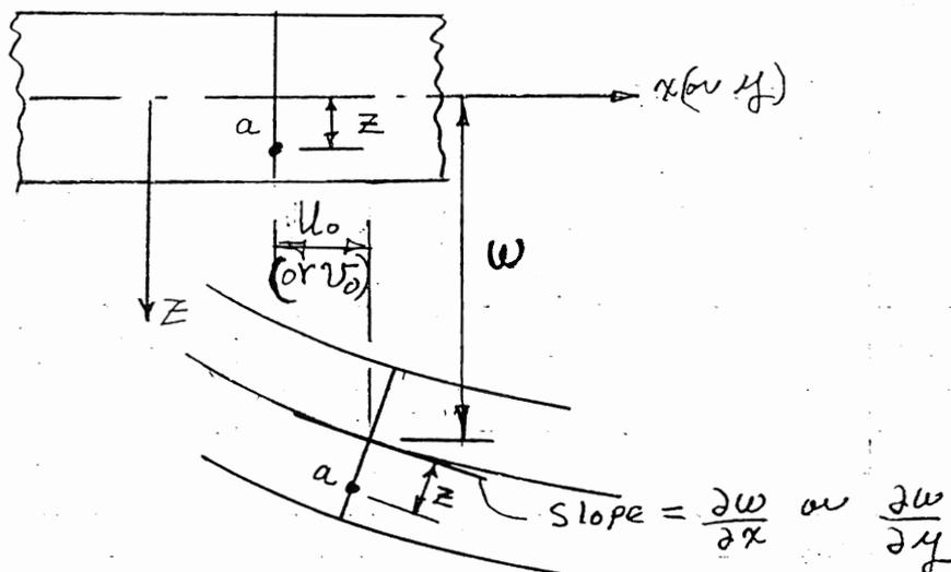
Displacement of Point (a) in "x" direction is given by
