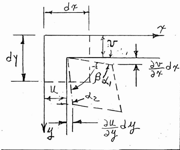
Shear strain  $\gamma_{ij}$  is defined as the angle change or distortion occurring within an element. Thus in the figure shown
