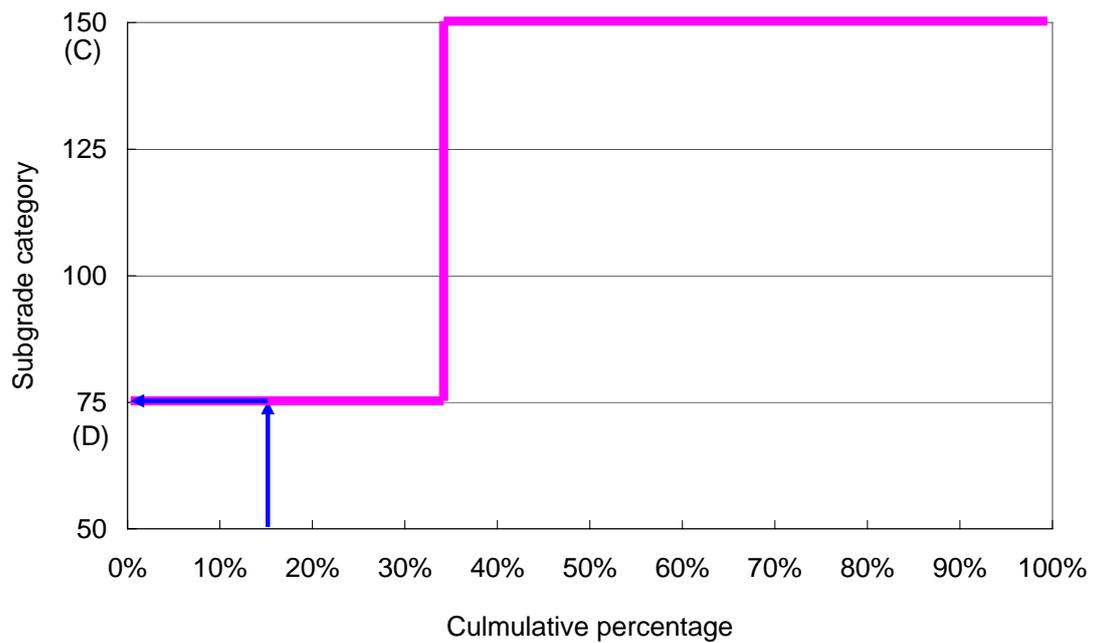
Figure 12 Subgrade Classes with Corresponding Cumulative Runway Length Percentage
