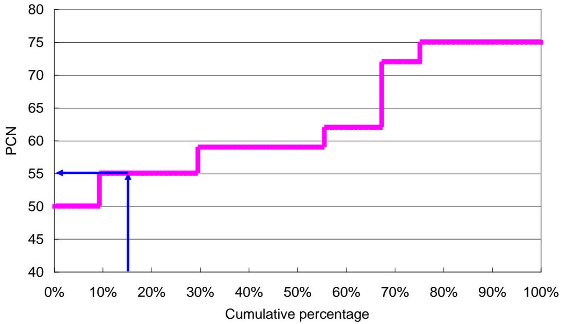
Figure 11 PCN Value with Corresponding Cumulative Runway Length Percentage
