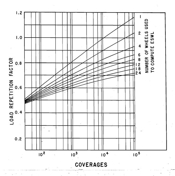
FIGURE 3. LOAD REPETITION FACTOR VS. COVERAGES
