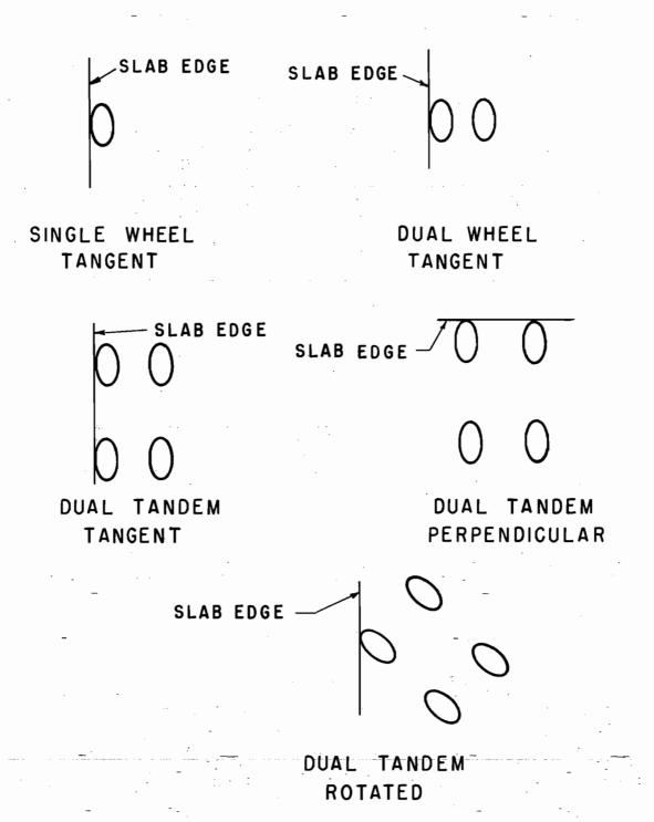
FIGURE 1. ASSEMBLY POSITIONS FOR RIGID PAVEMENT ANALYSIS
