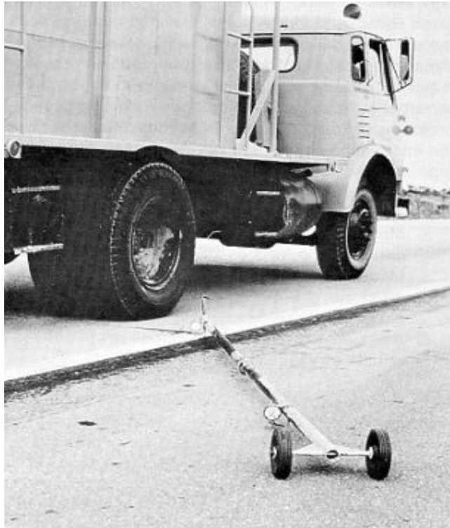
Figure 4-7.10. Device for monitoring slab lift. (23)
