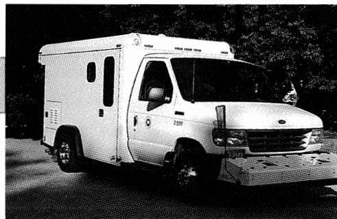
FIGURE 1. The Automatic Road Analyzer (ARAN) field-image/data-acquisition inspection system is used by the Connecticut Department of Transportation to assess the physical condition of state roads. The integrated system, which is installed in van-type vehicles (below), is equipped with lasers, accelerometers, gyroscopes, computers and camera boards, sensors, cameras, controllers, video-cassette recorders, and graphics cards. As the van is driven on the state roadways, the inspection system automatically maps and photologs imaging, positioning, and video data for workstation processing and analysis.
