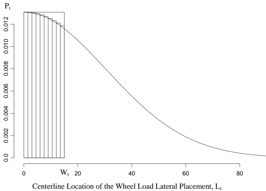
Figure 3 – Lateral Placement of the Centerline Location of the Wheel Load
