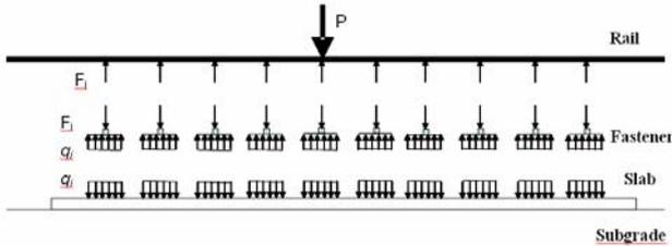
Figure 2. Illustration of the (a) substructures and (b) the free body diagrams of a slab track system.
