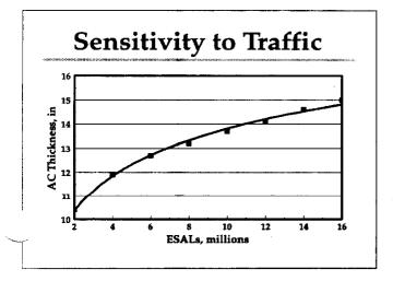
This is figure 2-1.7 (page 2-1.15), which illustrates the effect of traffic on the design thickness for a full-depth AC pavement.
