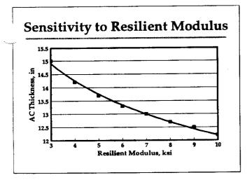
This is figure 2-1.8 (page 2-1.15), which illustrates the effect of the subgrade resilient modulus on full-depth AC thickness.
