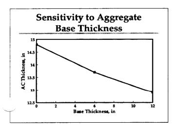
This is figure 2-1.10 (page 2-1.16), which illustrates the effect of aggregate base thickness on the AC thickness.
