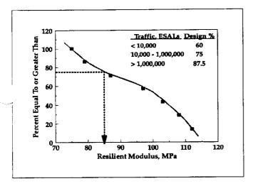
This is figure 2-1.2 (page 2-1.5), which illustrates how the design subgrade strength is selected.
