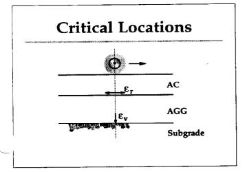
Vertical (compressive) strains on the subgrade are the cause of rutting. The procedure assumes a stable high-quality AC mix is used and rutting does not occur in the AC.
