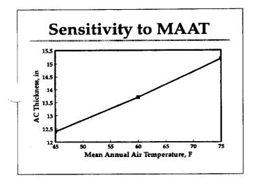
This is figure 2-1.9 (2-1.16), which illustrates the effect of the MAAT on full-depth AC thickness.
