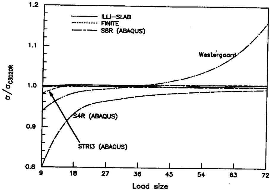
Figure 3-6 Stress comparison of interior loading
