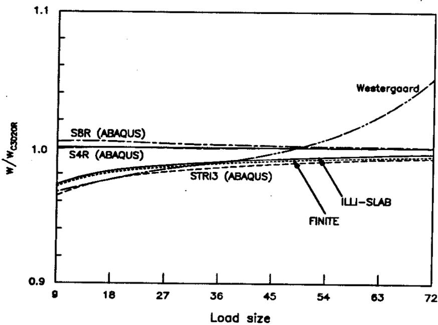
Figure 3-7 Deflection comparison of interior loading
