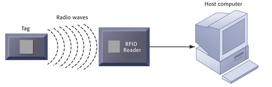
A microchip holds data including an identification number. The rest of the tag is an antenna that transmits data to a reader. Has an antenna that constantly transmits. When it senses a tag, it wakes it up, interrogates it, and decodes the data. Then it transmits the data to a host system over wired or wireless connections. Processes the data from the tag that have been transmitted by the reader.
