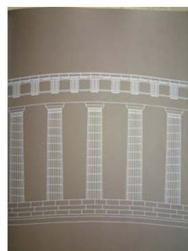
圖 29. The flat floor is not flat, but convex.
