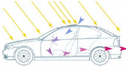
**Roof-operated Solar Ventilation**
