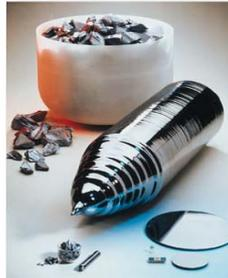
矽塊原材料、晶錠、晶片
