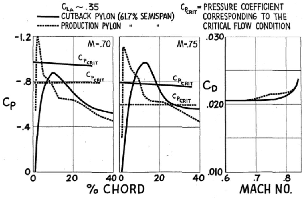
Pressure Coefficient in vicinity of outboard pylons of DC-8.
