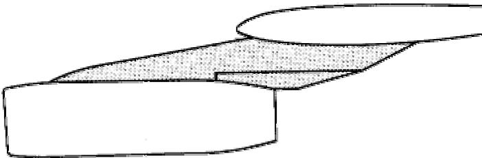
As engine bypass ratios have increased to about 6 - 8, this large gap is not acceptable. Substantial work has been undertaken to minimize the required gap to permit large diameter engines without very long gear.
