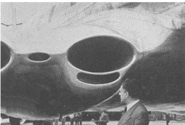
Wing-mounted nacelles can be placed so that the gas generator is forward of the front spar to minimize wing structural damage in the event of a disk or blade failure. Engine installations that do
