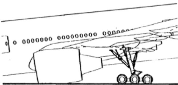
Current CFD-based design approaches have made it possible to install the engine very close to the wing as shown in the figure below. The 737 benefited especially from the closely mounted engines, permitting this older aircraft design to be fitted with high bypass ratio engines, despite its short gear.
