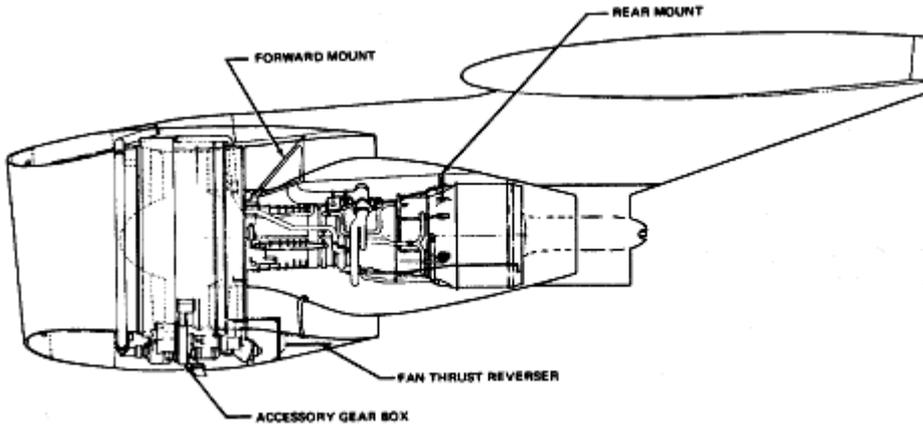
In the days of low bypass ratio turbofans, it was considered reasonable to leave a gap of about 1/2 the engine diameter between the wing and nacelle, as shown in the sketch of the DC-8 installation below.
