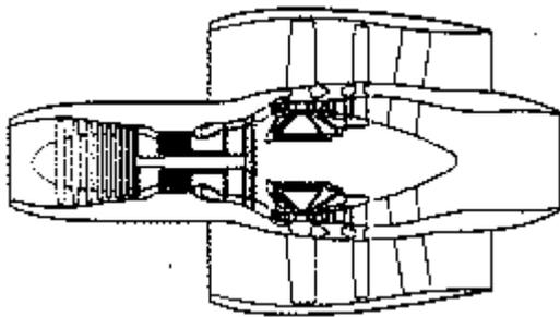
An unusual ADP with the fan located aft and attached directly to the turbine. Note the stator vanes in both turbine and fan sections to reduce swirl losses.
