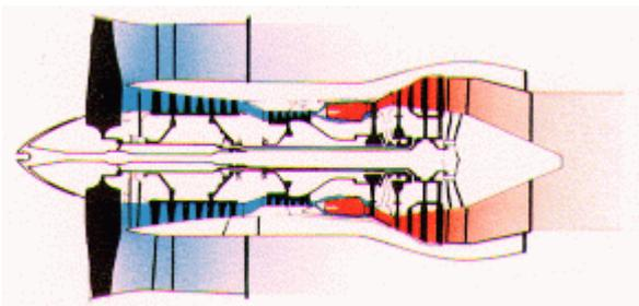
The figure below shows a Pratt and Whitney 4084 engine used on the 777. The diameter of this 84,000 lb thrust engine with nacelle is only somewhat smaller than the diameter of a 717.
