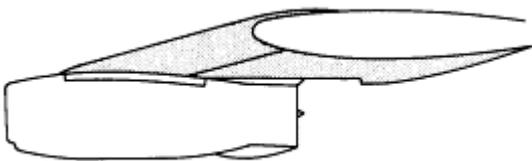
The original DC-8 pylon wrapped over the leading edge for structural reasons. Substantial improvements in  $C_{L_{max}}$  and drag rise were achieved by the "cut-back pylon" shown in previous figures. The figures below show the effect of this small geometry change on wing pressures at high speeds.
