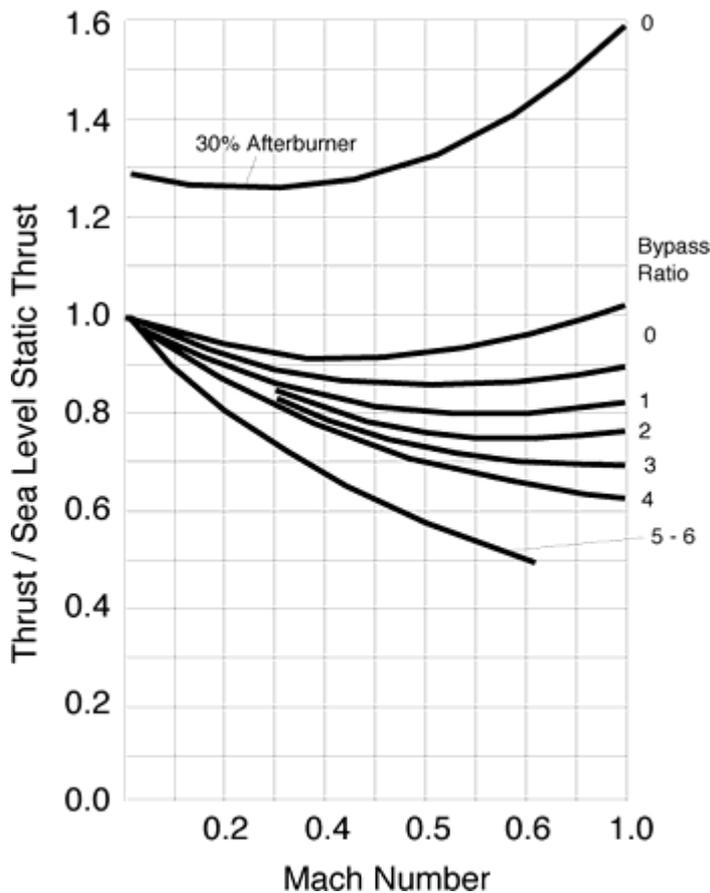
*Typical trend of thrust vs. speed for turbojets and turbofans with varying bypass ratio at sea level.*
