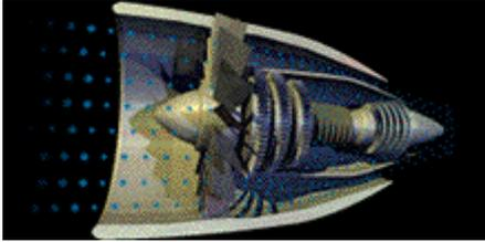
The operation of a propulsion system may be viewed simply as shown below. A fluid enters the system at speed  $V_0$  with a mass flow of  $dm/dt$ . It exits at speed  $V_e$ , and mass is added to the outflow at a rate  $dm_f/dt$ . The force exerted by this system includes the rate of change of momentum through the system and a pressure term:
