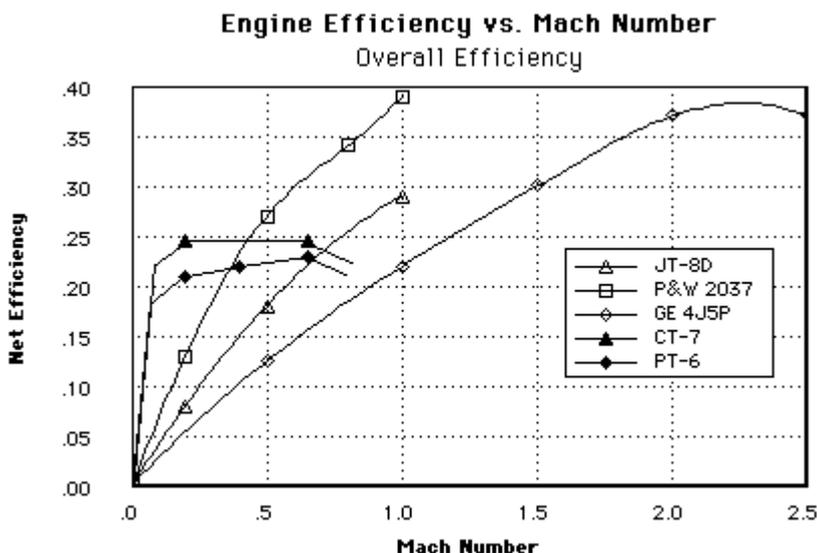
Overall efficiency of several engines vs. Mach number.
