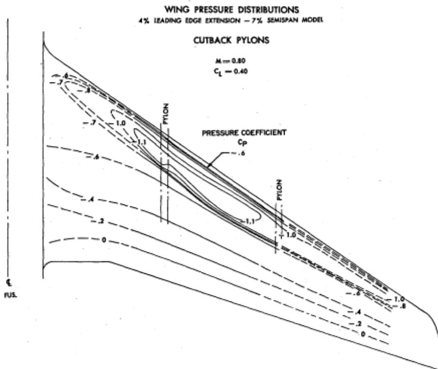
In addition, wing pylons are sometimes cambered and oriented carefully to reduce interference. This was tested in the mid 1950's, although the gain was small and many aircraft use uncambered pylons today.
