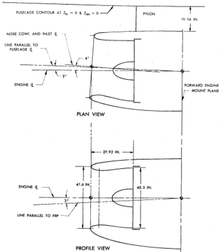
With an aft engine installations, the nacelles must be placed to be free of interference from wing wakes. The DC-9 was investigated thoroughly for wing and spoiler wakes and the effects of yaw angles, which might cause fuselage boundary layer to be ingested. Here efficiency is not the concern because little flight time is spent yawed, with spoilers deflected or at high angle of attack. However, the engine cannot tolerate excessive distortion.
