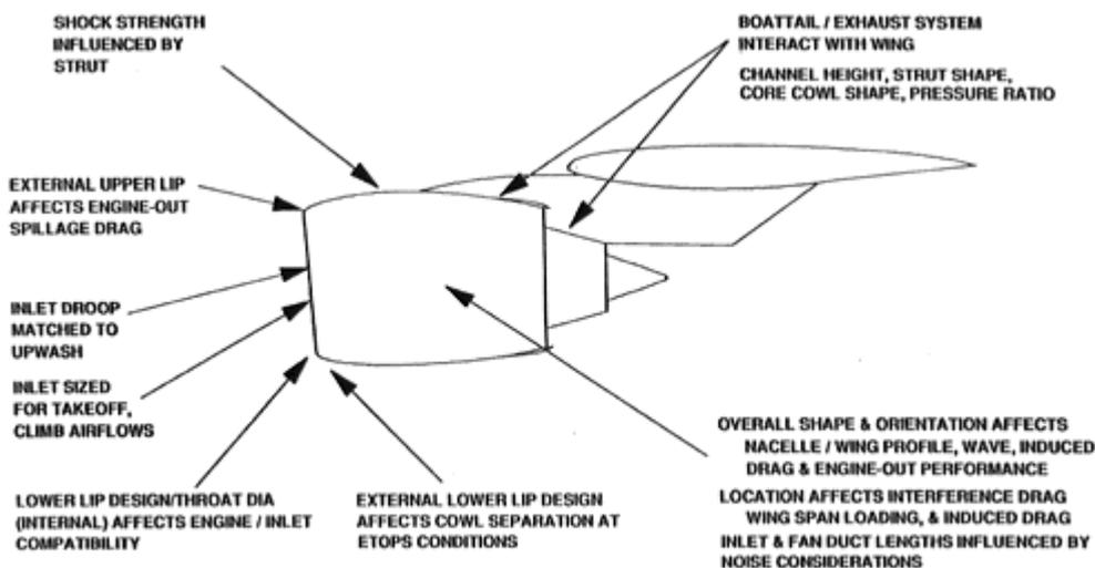
Some examples of nacelle designs and wing-mounted installations are shown below.
