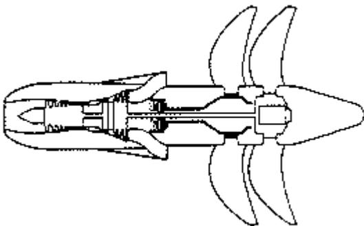
A counter-rotating prop-fan. At some value of bypass ratio, the advantages associated with the duct are overwhelmed by the weight and drag of the duct itself. Bypass ratio 50, ductless prop-fans such as the one shown here have been proposed for aircraft that fly up to Mach 0.8.
