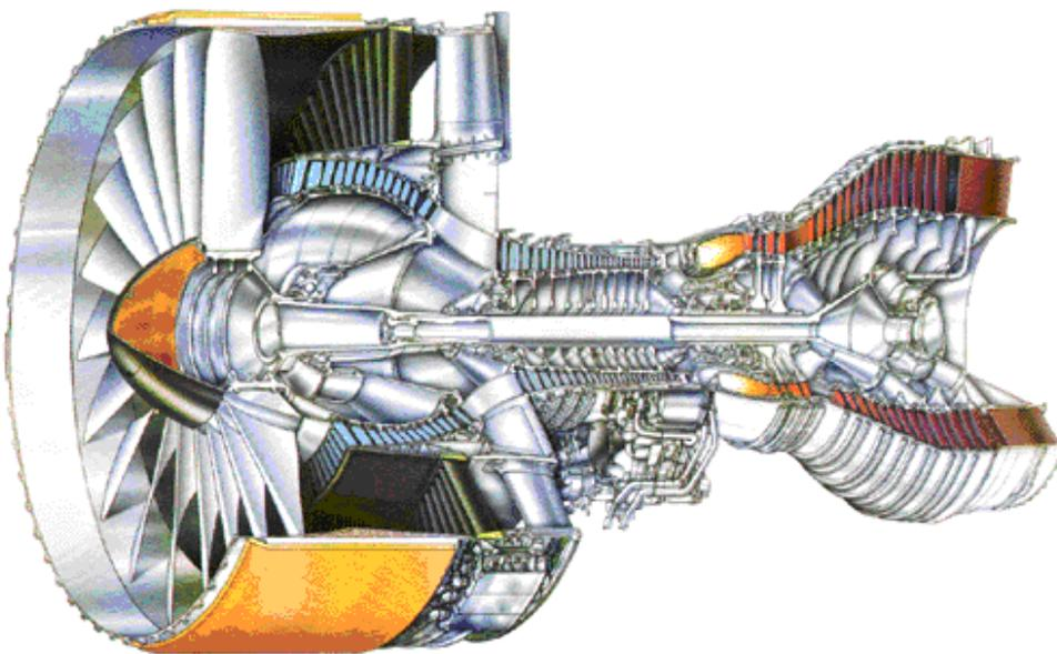
Cut-away showing the PW4000-Series of Engine
